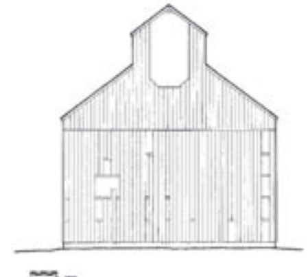
ROOF TYPE: MONITOR
